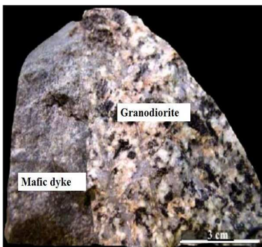
FIG.10-6. Mafic dike crosscutting granodiorite from the central part of the Elatsite porphyry deposit (after Strashimirov et al. 2003).
