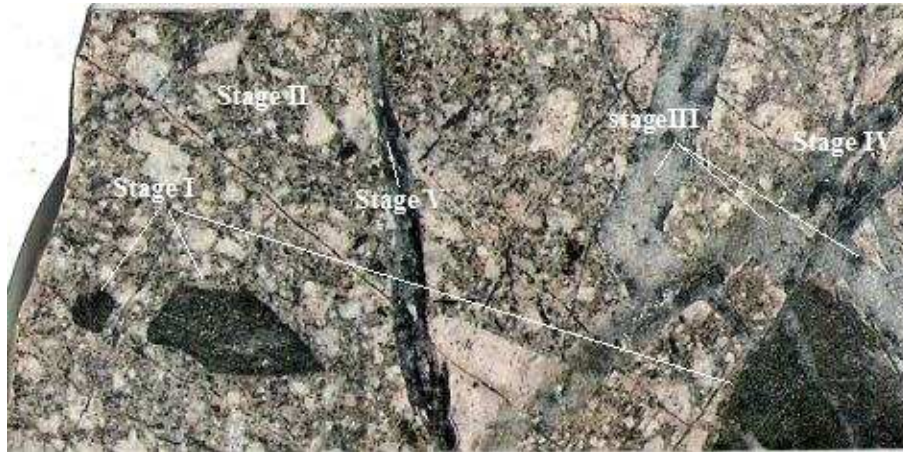
FIG. 10-2. Representative drill core sample of the Skouries Main monzonite porphyry (core width is about 4 cm), showing mineralization (disseminated and vein- type) in angular mafic fragments (stage I), pervasive (stage II), crosscutting relationships between successive quartz veins (stages III & IV) dominated by the magnetite-bornite-chalcopyrite assemblage, and a quartz-biotite vein (stage V), reflecting a range of hydrothermal evolution. The presence of mineralized mafic xenoliths within main porphyry is consistent with the multiple intrusive phases and mineralising events.
